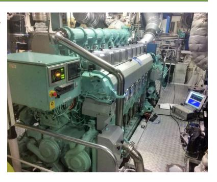
Rotational vibration measurement on flywheel and/ or shafts via speed pick-ups and/ or shaft encoder when;
